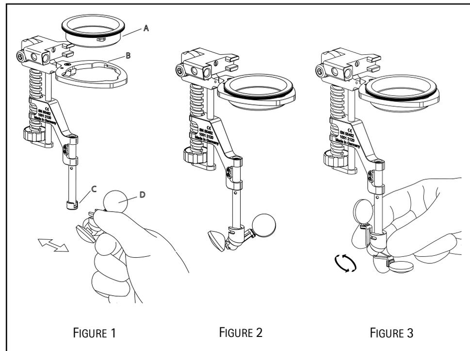
7. Using your thumb and index finger, hold the PIVOT Assembly as shown in Figure 1-D without touching the lens surfaces. **FAILURE TO HOLD THE CLIP IN THIS MANNER MAY RESULT IN DAMAGE TO THE ASSEMBLY.** Mount the PIVOT by inserting the black plastic tab into the slot (Figure 1-C).
